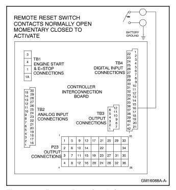
Figure 6-16 Remote Reset Switch Connections
